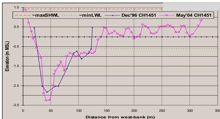
**Figure A1.15 Surveyed cross-sections through Goukou: Chainage 1451**
